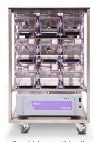
Completely compatible with modern high-density individually ventilated cage (IVC) rack systems capable of collecting spatial data for each individual animal at any given point in time.
