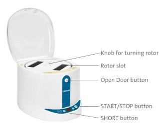
To avoid spillage of samples, only plates that have been heat or tape sealed should be placed in the centrifuge. Plates are loaded into the rotor in a vertical position.
